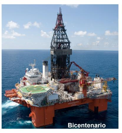
6th Generation Semisubmersible Drilling Rig, Design GVA 7500, four stabilized columns with capacity to operate in 10,000 ft. water depth and drill up to 35,000 ft. in moderated environment such as the Gulf of Mexico, West Africa and Brazilian Waters.
